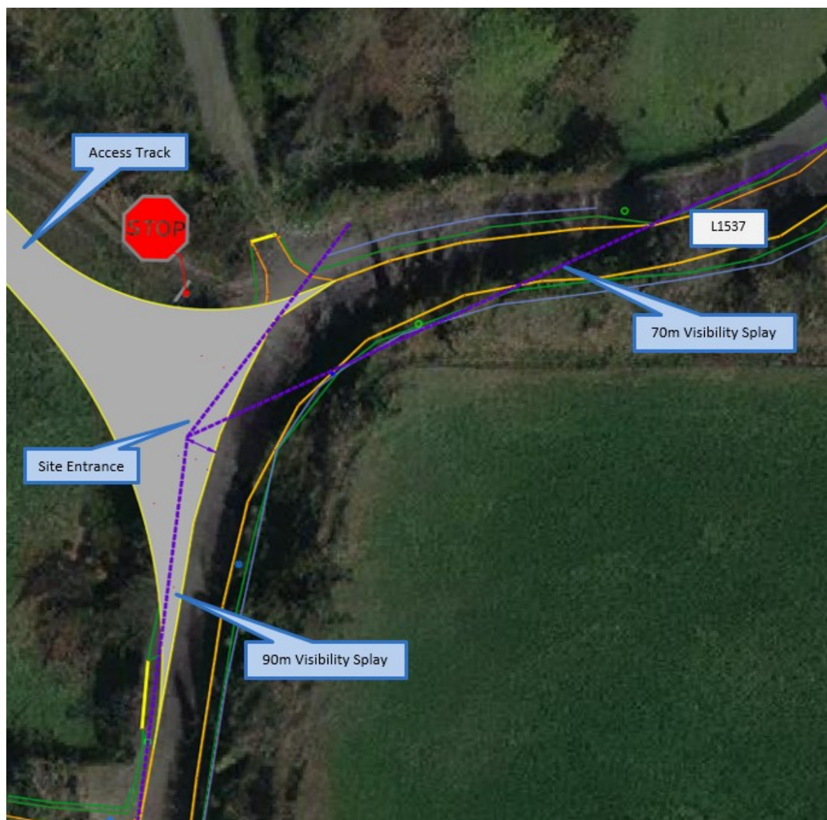
Plate 4 – Typical Site Entrance Upgrades
